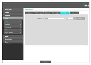
Product/ID: Specify the mounted pan/tilt driver's model and then set up an ID. Click Port and enter the pan/tilt driver's port speed, data bit, stop bit, and parity values as per the driver manufacturer's instructions.
