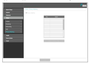
Privacy Masking Setup: Set up privacy masks (up to 16). Privacy masks are set up on Original View video. Thus, if video is dewarped, privacy masks are also dewarped.
