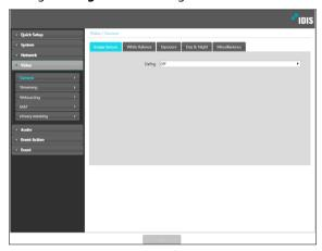
• **Defog:** Disables or enables the Defog feature. When it is enabled, image with a fog is adjusted.
