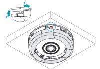
4 Slide the lens cover that surrounds the lens inside, then rotate the lens to adjust the focus.
