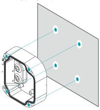
2 After wiring the cable, assemble the body to the bracket hinge. Tighten the screws of the hinge.
