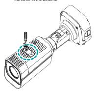
2 Instert a SD memory card into the SD memory card slot with the 'micro SD' print facing upward.
