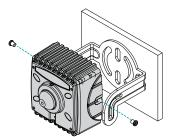
2 Adjust the angle of the camera module.
