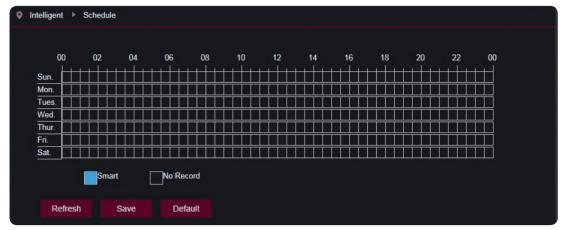
One cell in the table is 30 minutes. In the scheduled time, recording will be stored into the SD card when an event of detection setting (PID, LCD, SOD, FD or CC) is occurred.
