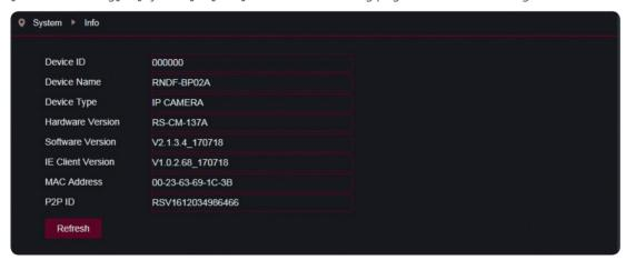
Displays the system information of the device, including device type, MAC address and software version.
