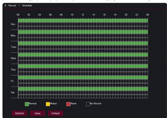
One cell in the table is 30 minutes, first line is normal record, second line is motion detection alarm, third line is alarm record. User can setup according to private requirement to choose different record type and time.
